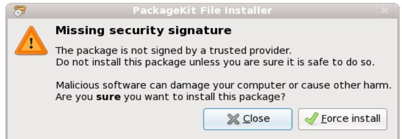
Fig. 7. Forcing the RPM installation
